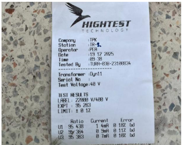
VOLTAGE TURN RATIO TEST
