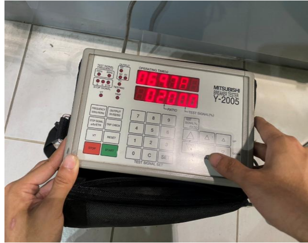
ACB TRIP UNIT TEST
