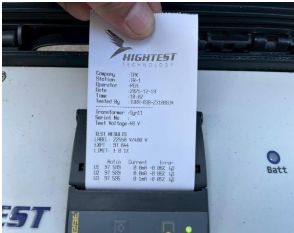
VOLTAGE TURN RATIO TEST
