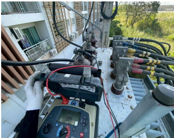
INSULATION RESISTANCE TEST
