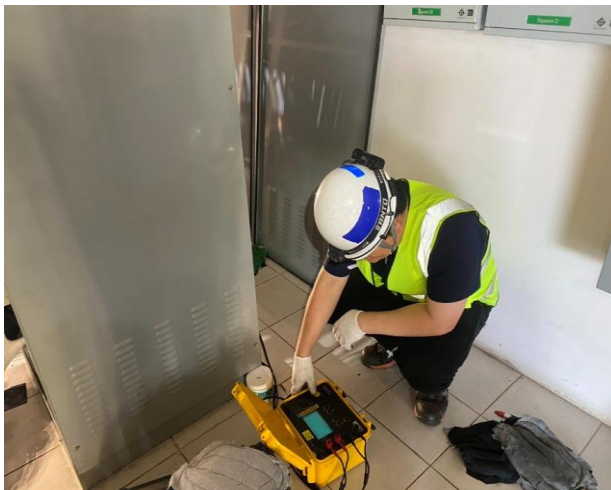
CONTACT RESISTANCE TEST
