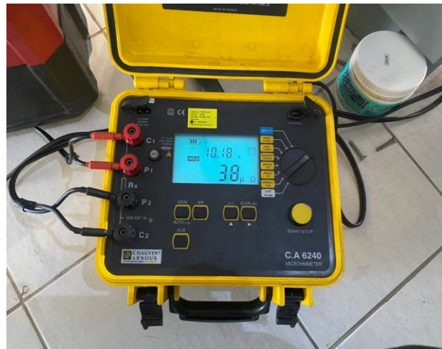
CONTACT RESISTANCE TEST
