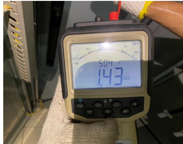
INSULATION TEST
