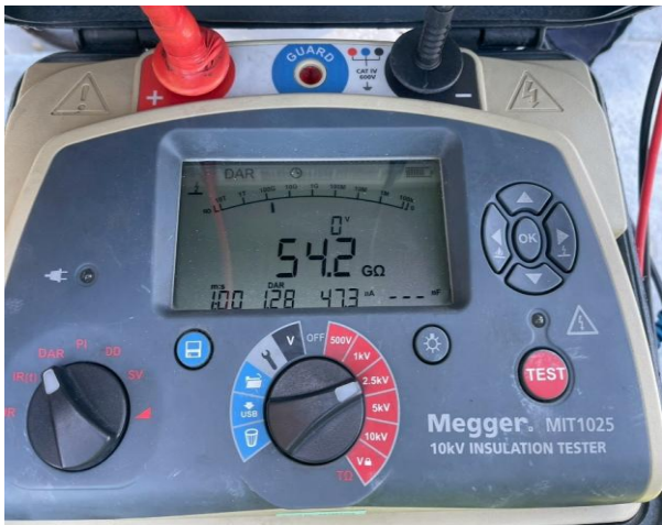
INSULATION RESISTANCE TEST
